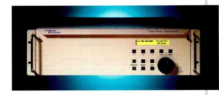
The Time Machine is a new, technological break through product, which reduces program time, to create commercial insertion time. it is a self contained, small 3U rack mountable unit which requires no data compression.
