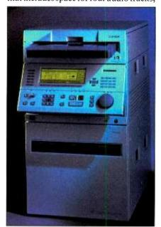
This D-6 recorder from Philips offers uncompressed high-definition recording on a D-1-sized cassette.
