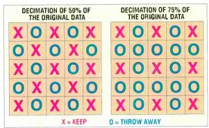
As part of many compression processes, images are first decimated, depending on the compression scheme, various amounts of data are simply thrown away. During decompression, pixels that were thrown away are regenerated using interpolation. If, for any reason, an image is shifted by a single pixel, the next decimation could remove all that is left of the original data.
