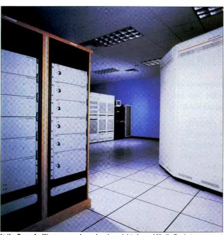
In the Speer facility, a seven-channel and an eight-channel Media Pool store content required for real-time playback.
