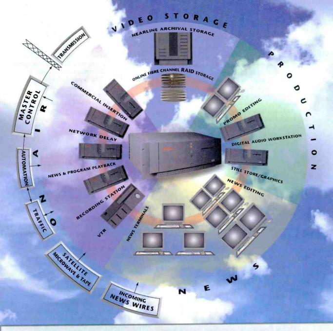
ASC's VR300™ Broadcast Video Server is more flexible, more scalable, and more reliable. With 1,066 Mb/sec available bandwidth, it provides up to 24 simultaneous channels and 96 hours of online digital storage.
